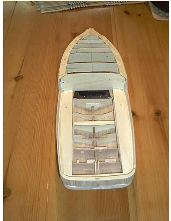
Solid balsa bow (below) allows me to tool it into a variety of shapes.
