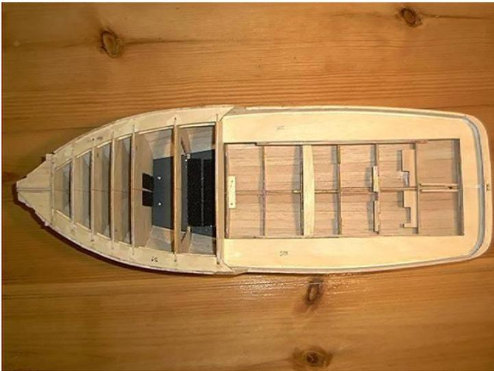
Same ash and balsa plywood hull and strip plank construction as the Three Sons. Black subdeck (above) holds six C and four AA batteries for the motor, radio control, running lights and radar turret power. What I like about this sturdy little \$99 model is that it be customized into a variety of tugs and trawlers. Seems like every model builder thinks so too because Dumas is always out of stock. Ironic that Dumas Products is located in Tucson – the middle of the desert.
