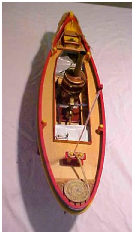
Hull is one-piece formed polyurethane – like really thin sprinkler pipe.
