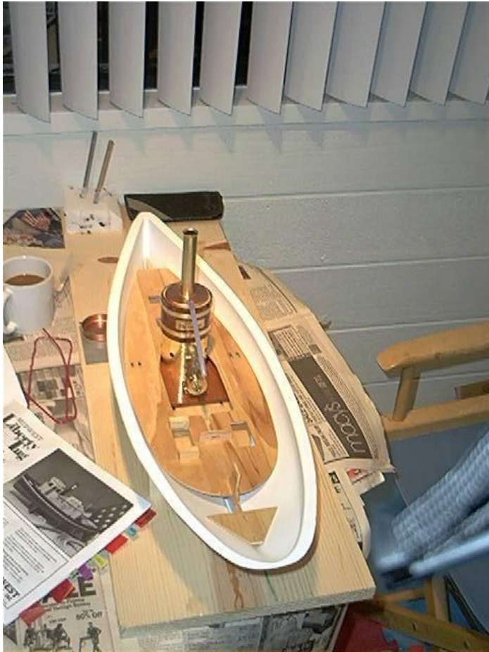
Hull is one-piece formed polyurethane – like really thin sprinkler pipe.
