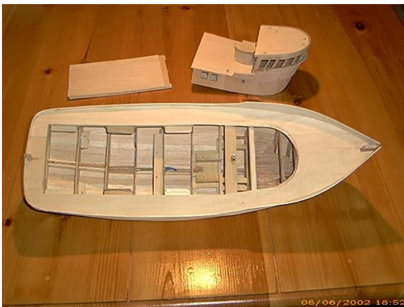
Built like the real thing! Hull planks made from 1/8" x 1/2" balsa – one plank at a time...
