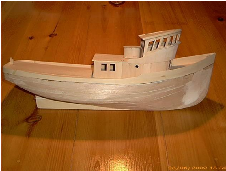
Subdeck made from 3/32" ash ply. Top deck made from 1/16" scored ash.
