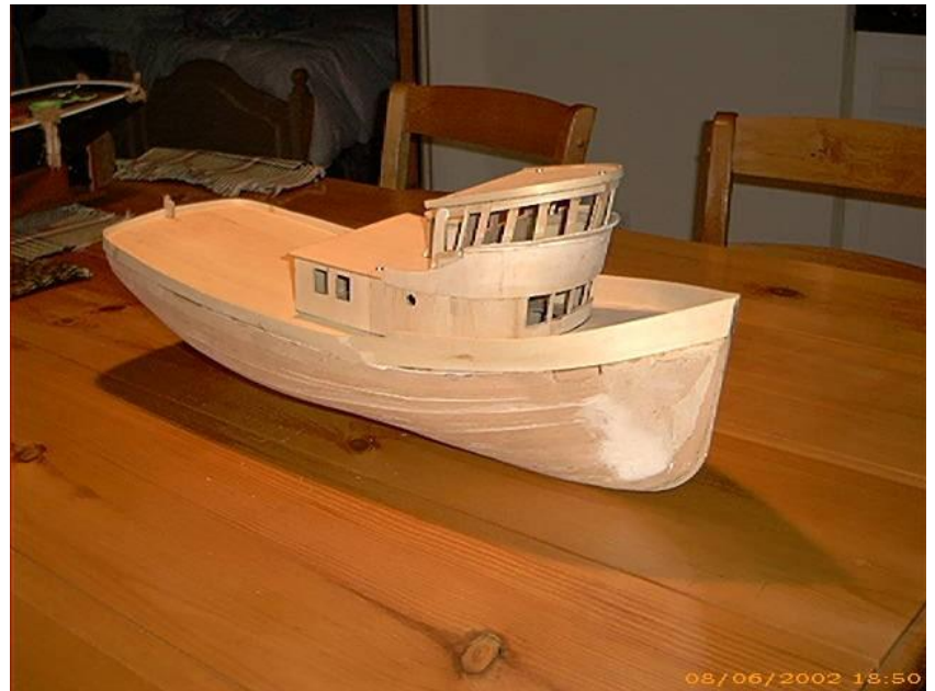
Subdeck made from 3/32" ash ply. Top deck made from 1/16" scored ash.
